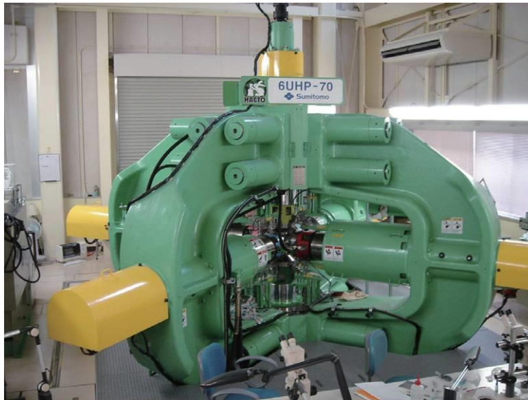
Fig 3.1.1 A 6-rams-LVP at the Institute for Study of the Earth's Interior, Okayama University.
